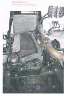
MAN-Motor: 1150 PS/6000 Nm
